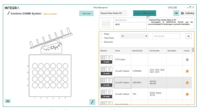
In the labware library, the Slanted Plate Holder (20°) is assembled e.g. with a 24 well plate.
