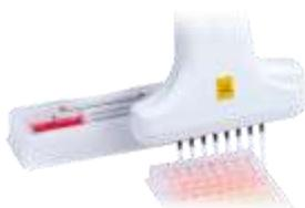
The divided reservoir is designed to be compatible with all VIAFLO fixed spacing and VOYAGER adjustable tip spacing multichannel pipettes. For example, the 12.5 and 125  $\mu\text{l}$  8 channel VOYAGER adjustable tip spacing pipette compressed to 4.5 mm spacing can access the 5 ml reservoir compartment and then expand to 9 mm spacing to access a 96 well plate.
